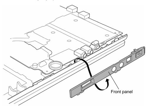
Figure 4-30 Removing the front panel
